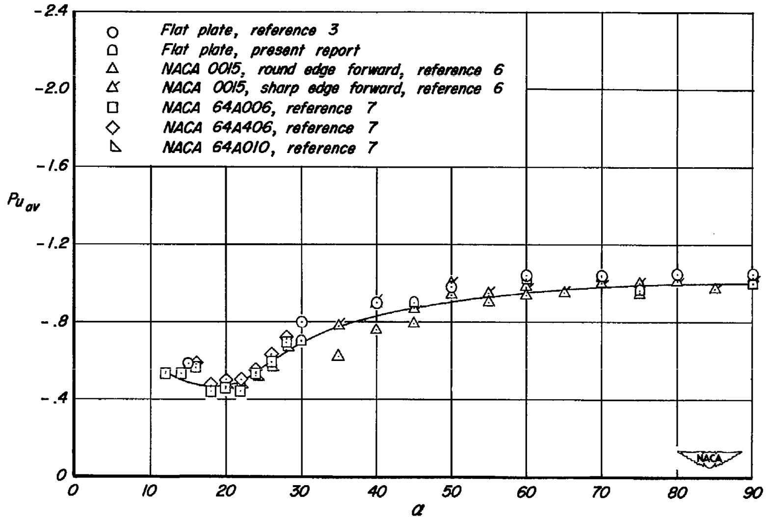
Figure 5.- Average upper-surface pressure coefficients on plates or airfoil sections with completely separated upper-surface flow.
