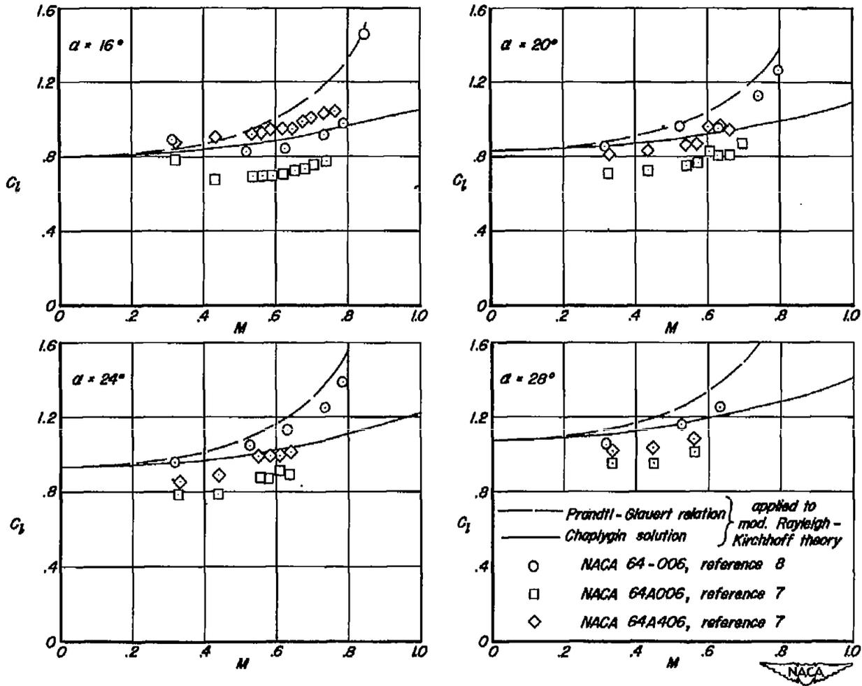
Figure 7.- Comparison of the measured effects of compressibility on the lift characteristics of several thin airfoil sections at high angles of attack with the effects predicted for a flat plate by applying either the Prandtl-Glauert relation or the Chaplygin solution to the modified Rayleigh-Kirchhoff theory.
