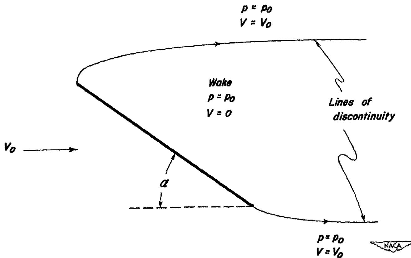
Figure 1.- Flow about an inclined flat plate of infinite span, as assumed in the Rayleigh-Kirchhoff theory.
