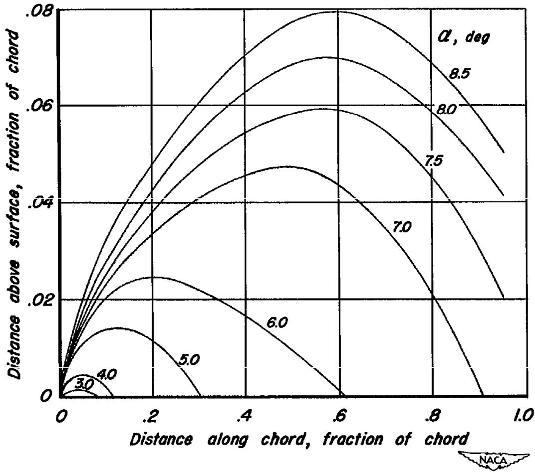
Figure 4.- The extent of upper-surface flow separation on a faired double-wedge airfoil section (ref. 4).
