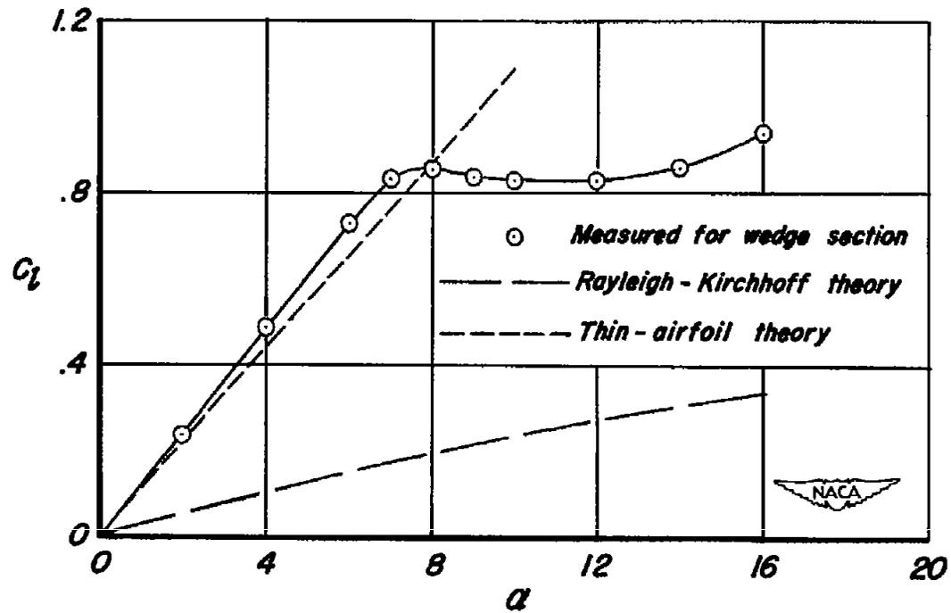
Figure 3.- Comparison of the measured lift characteristics of a faired double-wedge airfoil section (ref. 4) with lift characteristics given by the Rayleigh-Kirchhoff theory and by thin-airfoil theory.
